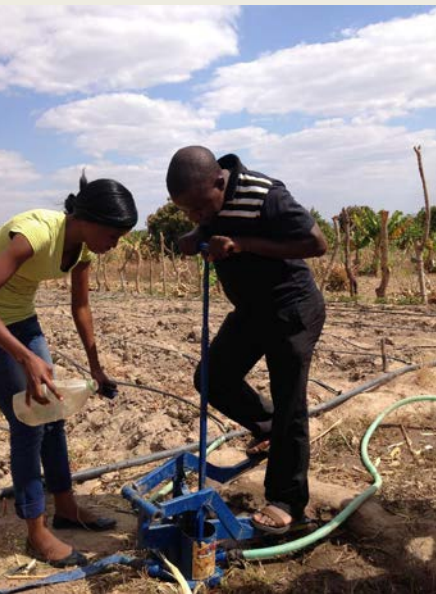
Photo: Learning to use the treadle pump. M. Messner 2015
