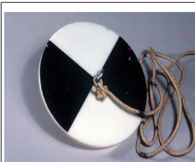
Figure 4: Secchi disk for measuring transparency
