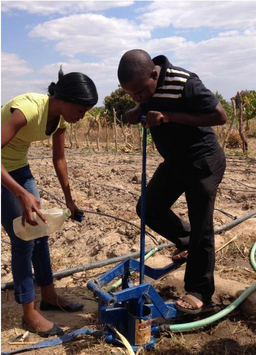
The treadle pump reduces the difficulty of irrigation. © M Messner 2015
